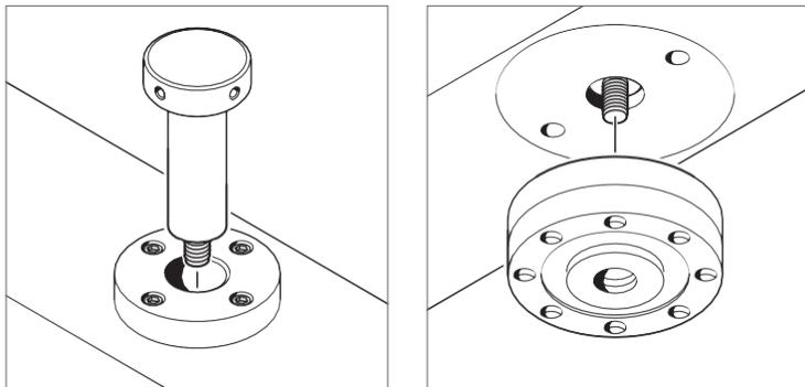
Place the adapter into the moving crosshead... then screw the adapter into the load cell.
