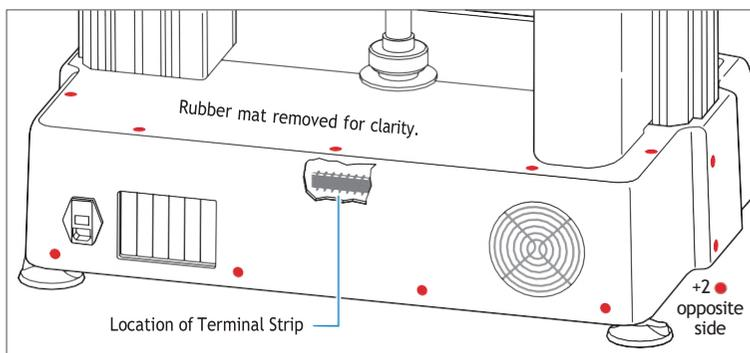
Remove the 13 screws (●) to remove the rear plastic housing shroud...
