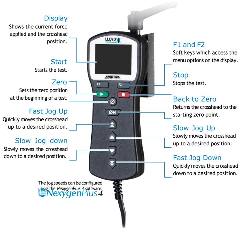
The jog speeds can be configured using the NexygenPlus 4 software.
