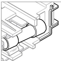
**Note:** The fuses must be installed with one end touching the pin end of the fuse holder.
