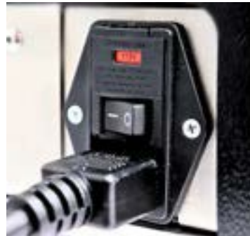
The Main Power switch.
