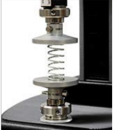
Proper alignment of the test specimen.
