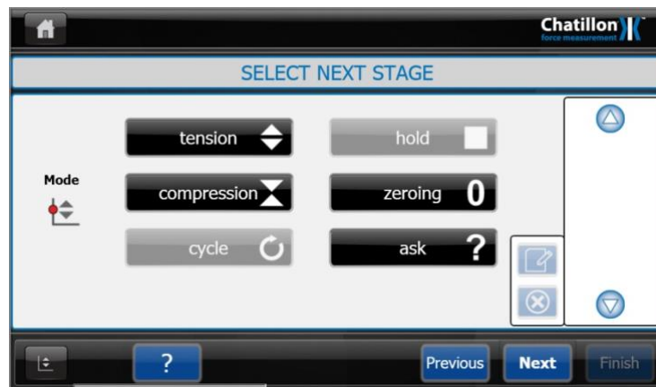
The Icon at the left-hand side of the screen shown above shows "Normal Mode" (Red dot halfway up the vertical line).
